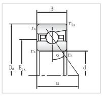
MONTON B719XX extremely light Series Angular Contact Ball Bearings diameter from 10-670
