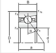
MONTON B72XX robust Series angular contact ball bearings size from10mm-400 mm.
