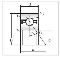
MONTON B72XX robust Series angular contact ball bearings size from10mm-400 mm. B72 series bearings have a large
