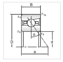
MONTON B70XX light series angular contact ball bearings are inseparable design, produce size range inner diameters from
